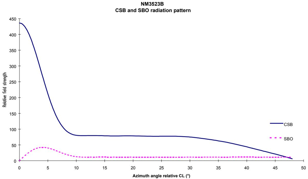
**Figure 5-7 CSB and SBO radiation patterns including LPDA**
