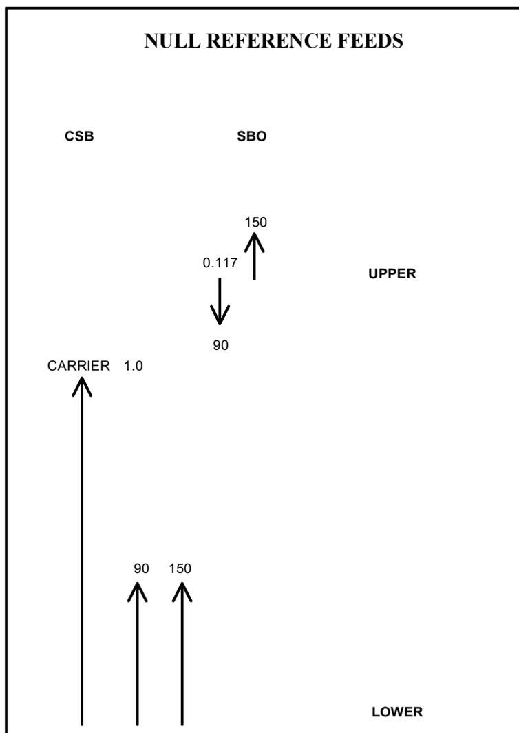
**Figure 6-5 Vector representation of Null-Reference feed signals**
