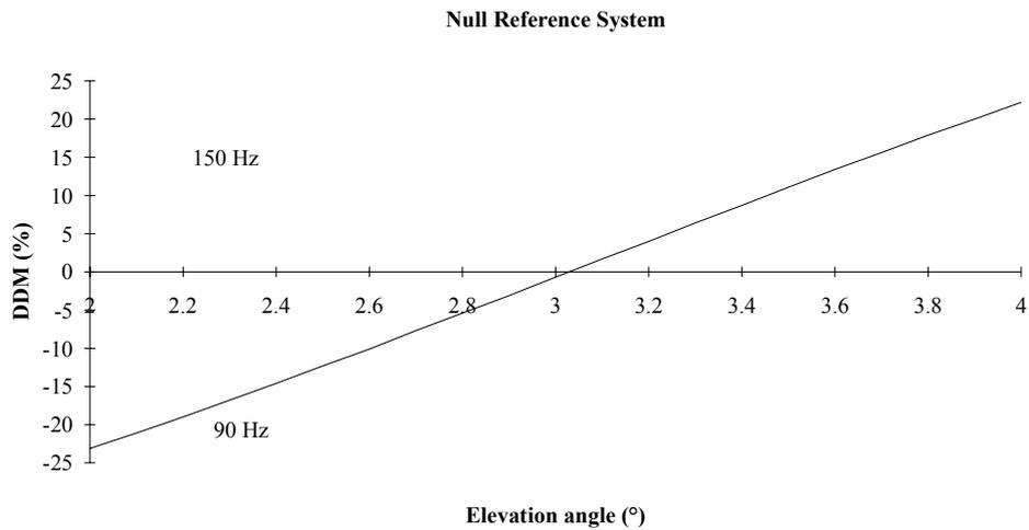
**Figure 7-5 DDM distribution at 62 m from the antenna system**
