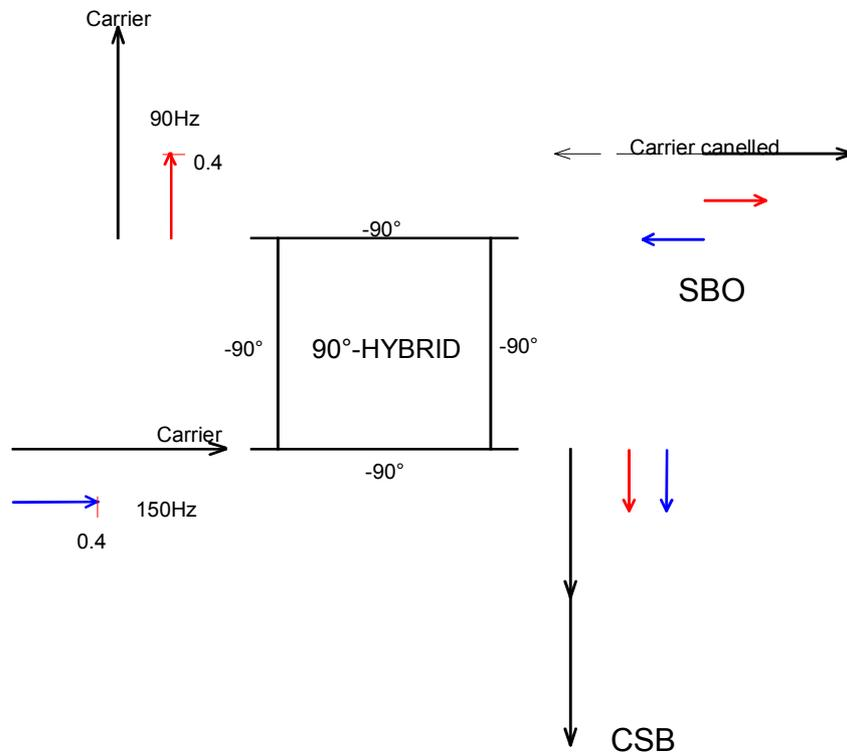
**Figure 2-18 CSB and SBO generation in a Quadrature Hybrid in NM7000 Transmitter**
