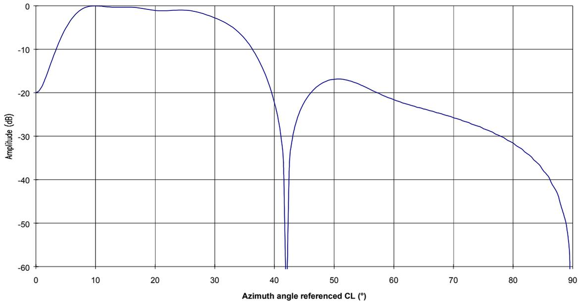
**Figure 5-19 CSB Clearance lobing (dB)**
