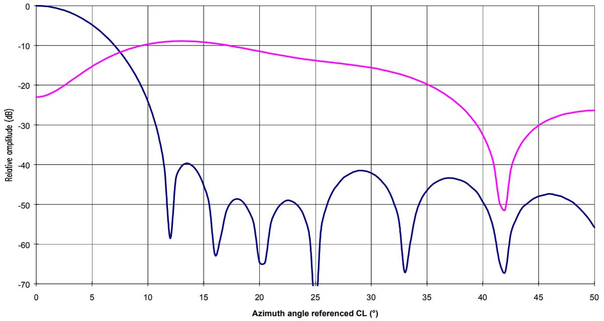
**Figure 5-10 Antenna Course and Clearance lobing**
