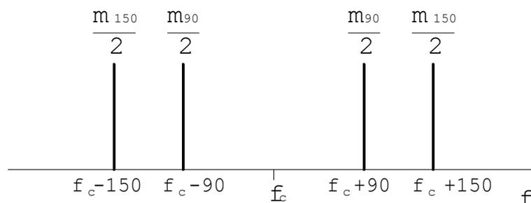
**Figure 2-7 Frequency spectrum of a DSB-SC signal modulated with 90 Hz and 150 Hz (SBO)**
