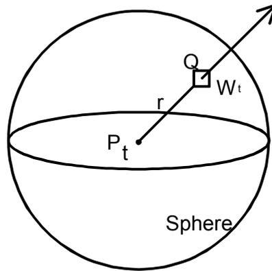
**Figure 3-6 Radiation of the Power  $P_t$  from an Isotropic Radiator**
