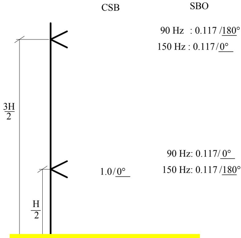
**Figure 6-6 Sideband Reference Antenna Configuration**
