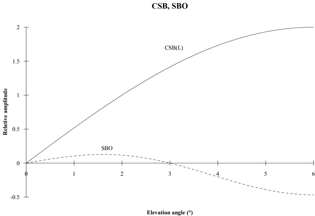
**Figure 6-7 CSB and SBO lobe pattern for Sideband Reference Antenna system**
