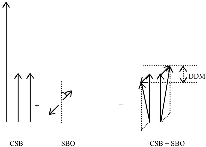
**Figure 2-11 Phasing error between CSB and SBO. SBO is retarded by  $\phi$  degrees**
