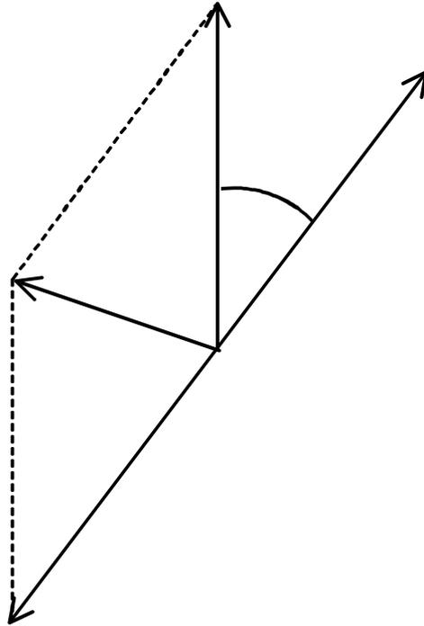
**Figure 3-15 The phasor signals from an antenna above ground plane and the image antenna**
