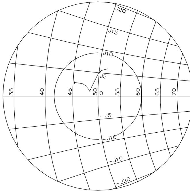
**Figure 4-8 Typical impedance characteristics of a localizer antenna element**
