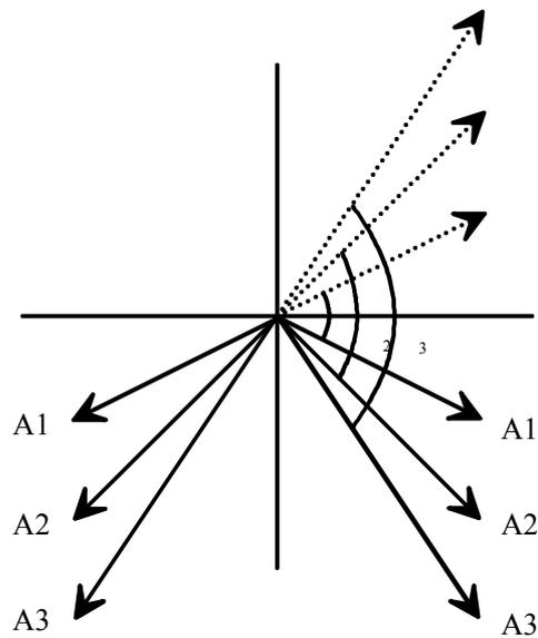
**Figure 3-13 The radiation vectors for an antenna array of six elements with three of the elements fed 180° out of phase**
