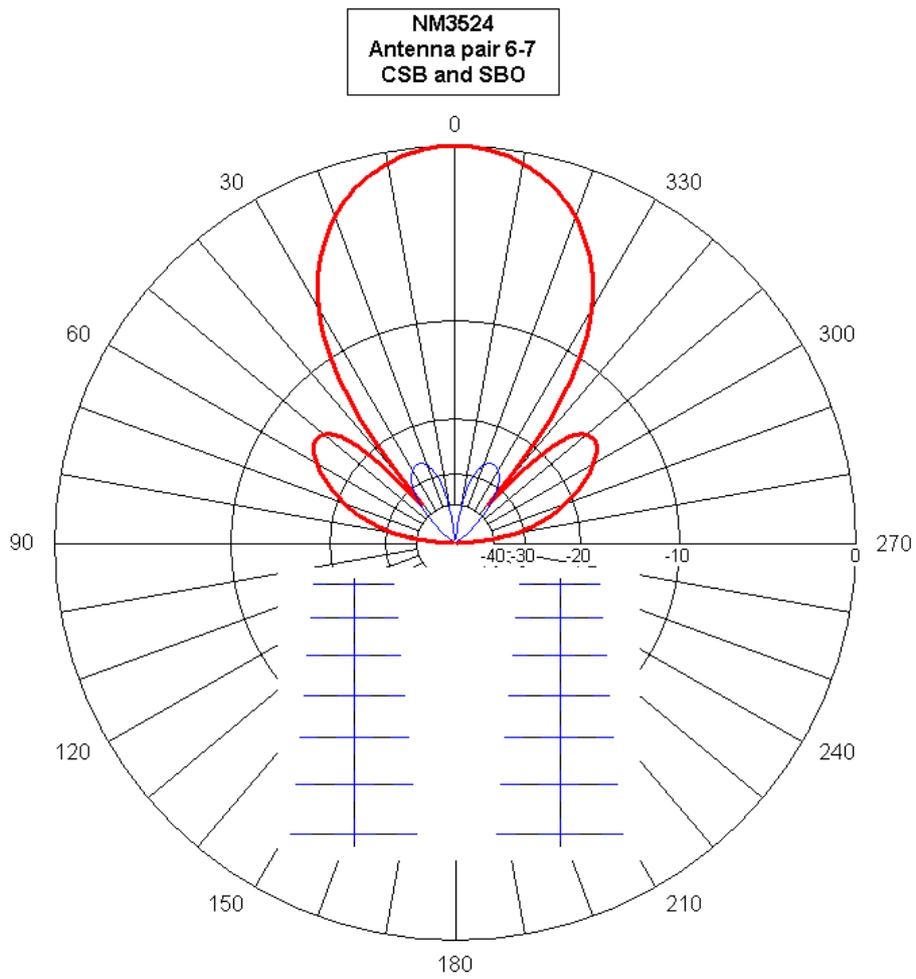
**Figure 5-11 Polar diagram of CSB and SBO lobing from one antenna pair**
