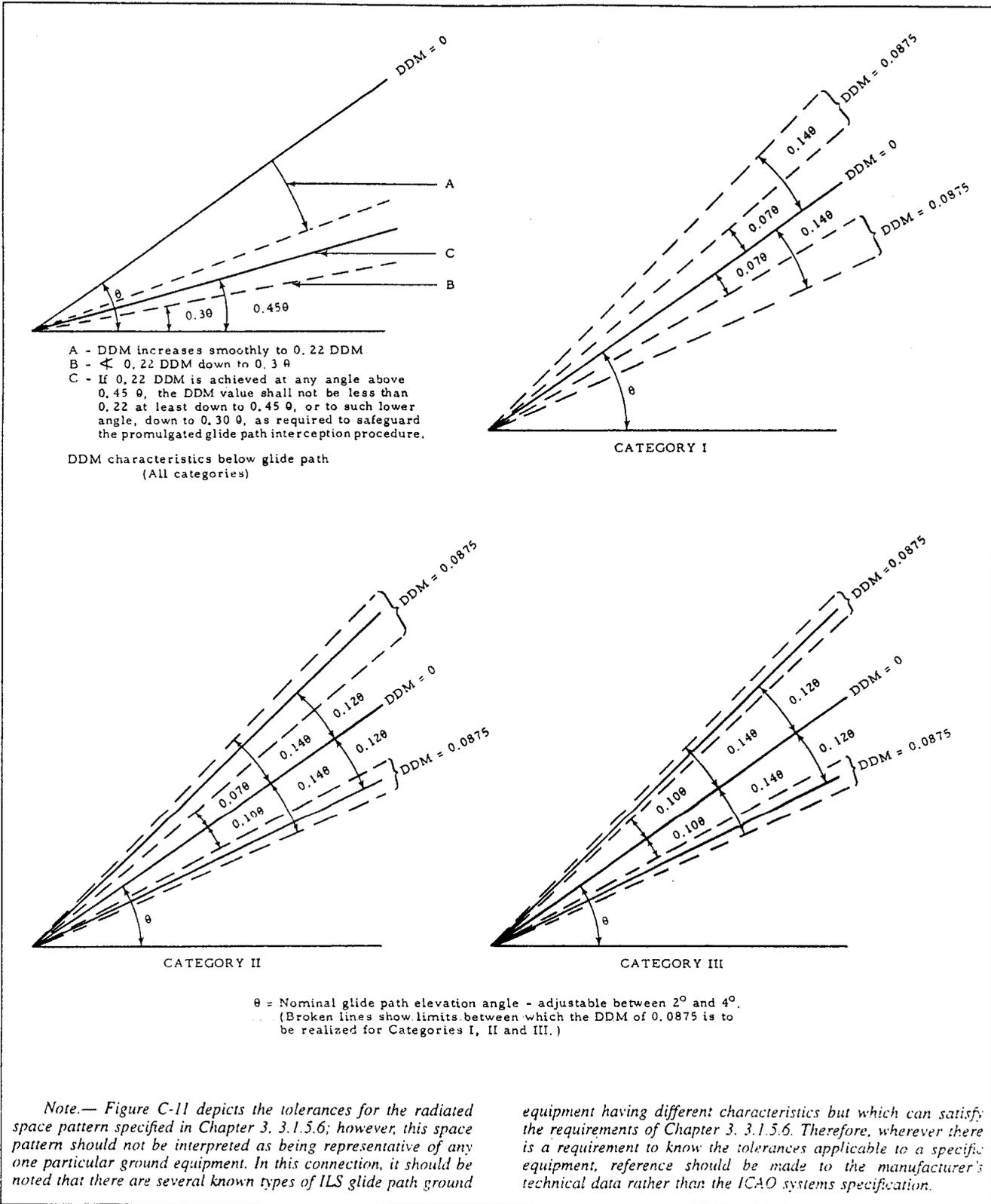
Figure C-11. Glide path — difference in depth of modulation
