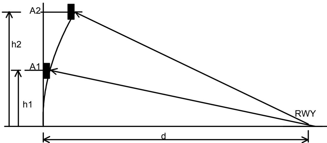
**Figure 6-18 Geometric illustration of antenna element offset**
