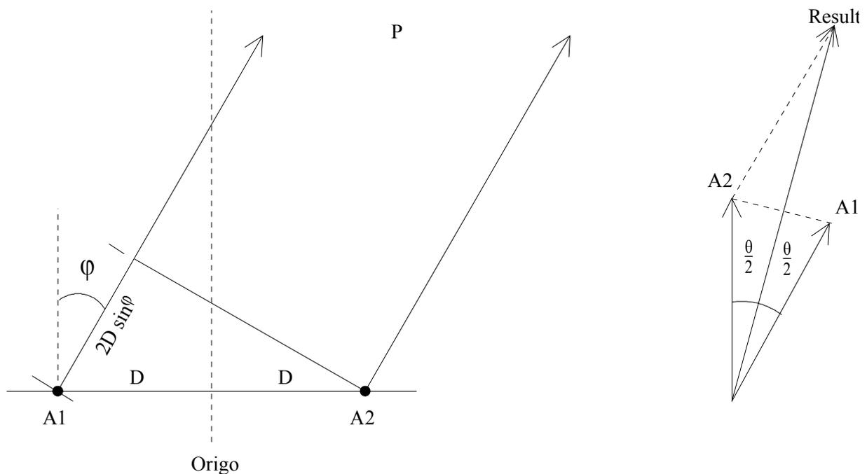
**Figure 3-9 Path delay between two antenna elements**
