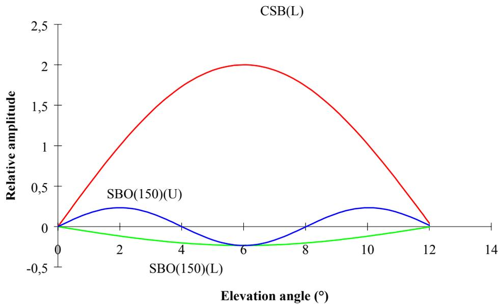
**Figure 6-8 CSB and SBO element radiation pattern for Sideband Reference system**
