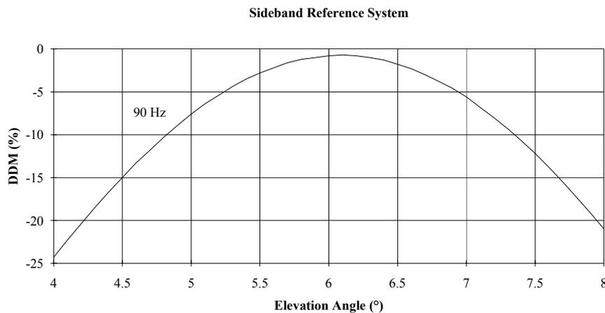
**Figure 7-6 DDM distribution at 42 m and 6° elevation**
