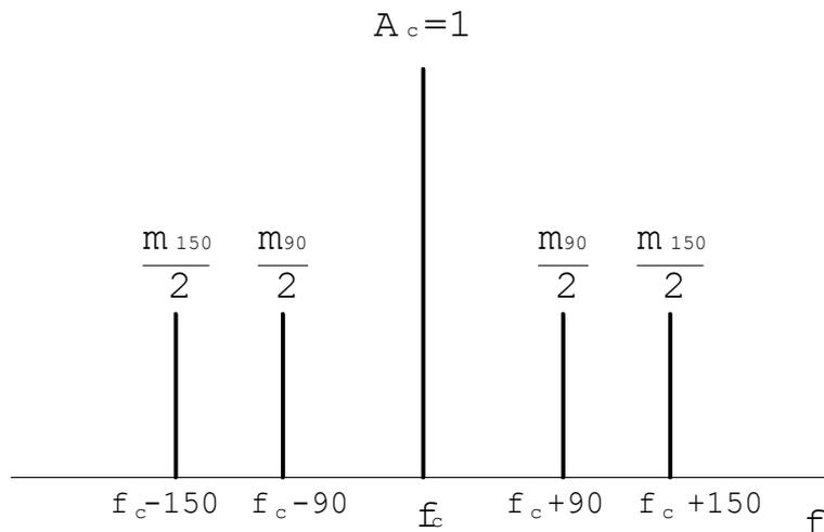
**Figure 2-5 Frequency spectrum of a AM signal modulated with 90 Hz and 150 Hz (CSB)**
