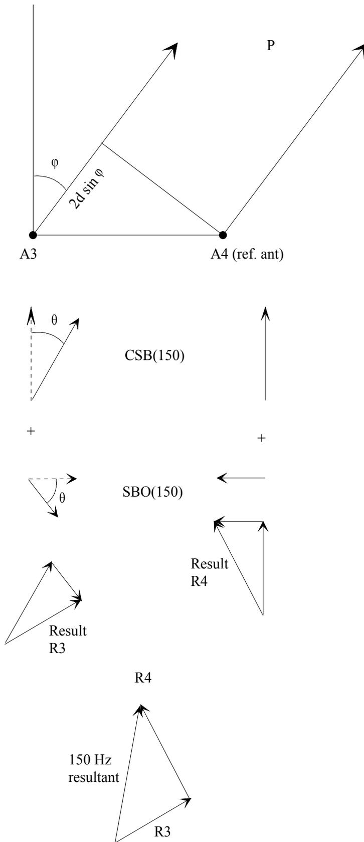
Figure 4-2 Resulting 150 Hz sideband from two-antenna feeds
