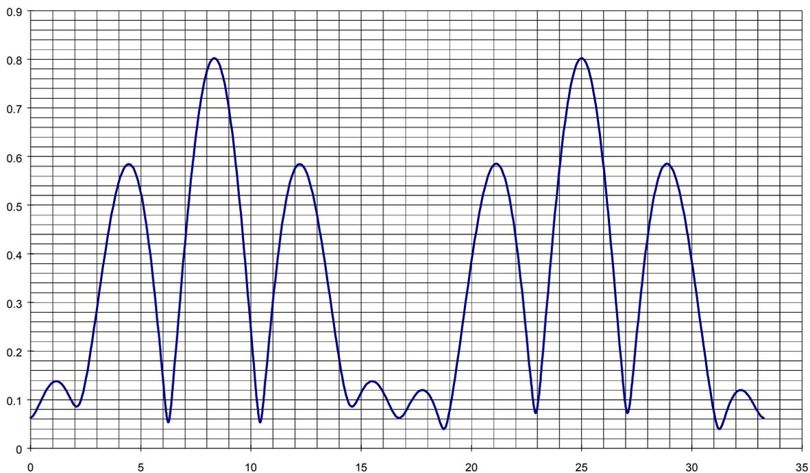
**Figure 2-20 Demodulated SBO with 3.6° internal phasing error corresponding to -30 dB carrier residual**
