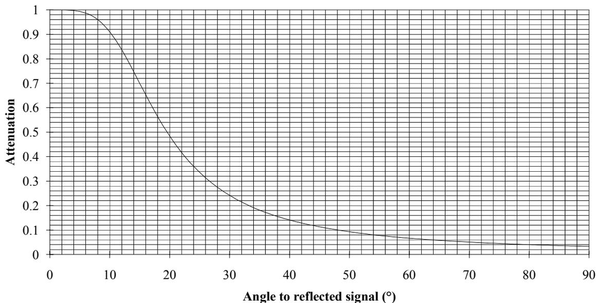
**Figure 8-4 Attenuation of localizer beam bends caused by the aircraft ground speed of 105 knots**
