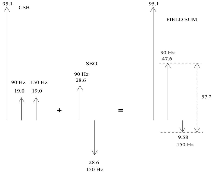
In the **field sum** the 150 Hz modulation components is 180° out of phase with the 90 Hz because the SBO amplitude is larger than the modulation level of the CSB.
