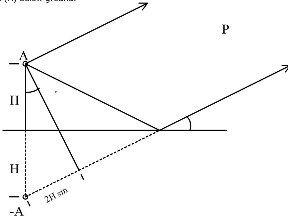
**Figure 3-14 Horizontally polarized antenna above ground plane**
