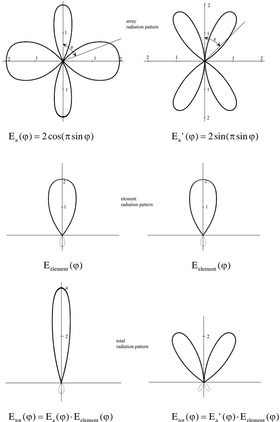
**Figure 3-11 Radiation patterns of two antenna elements spaced  $d = \lambda$ :
