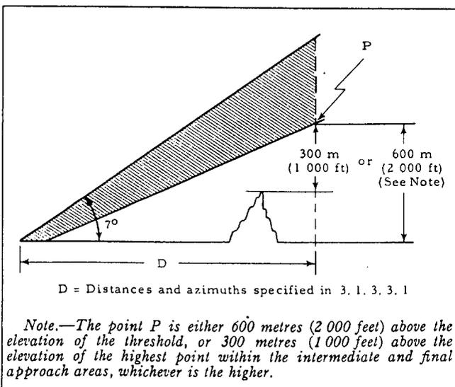
Figure C-8. Localizer coverage with respect to elevation
