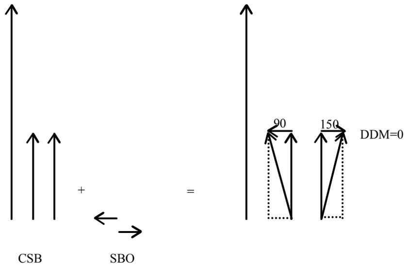
**Figure 2-12 CSB and SBO in quadrature. (90° phase)**
