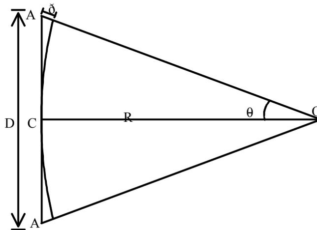
**Figure 3-2 Calculation of the extent of near field with an acceptable phase error ( $\lambda/32$ ) from an antenna of length D**
