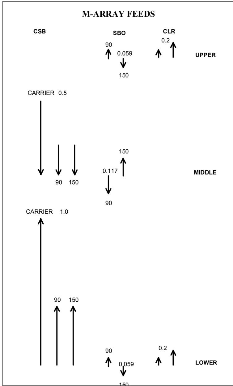
**Figure 6-16 Vector representation of M-Array feed signals**
