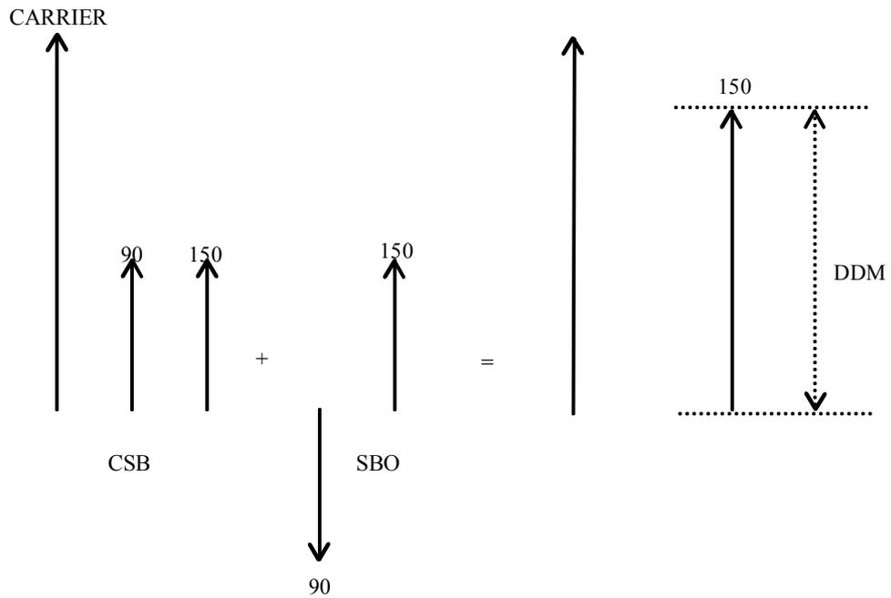
**Figure 2-13 SBO amplitude is equal to CSB modulation depth**
