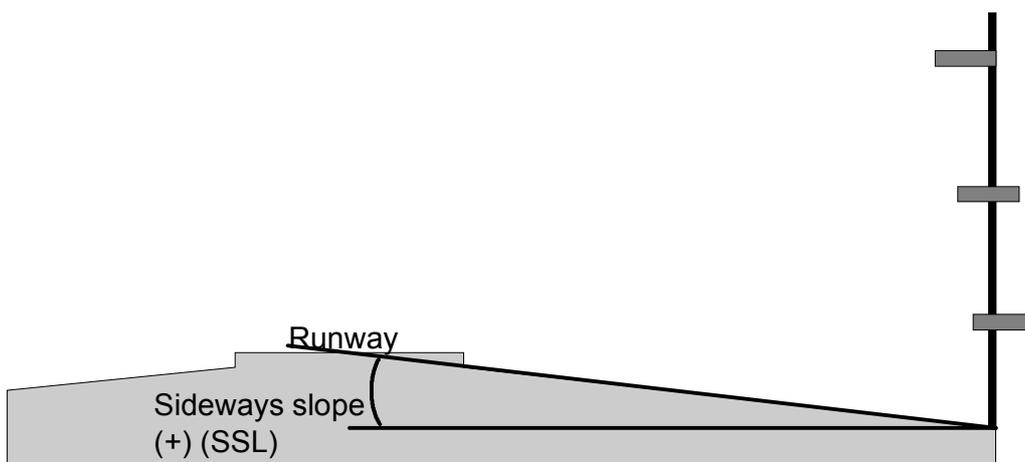
**Figure 6-20 Definition of Sideways Slope (SSL)**
