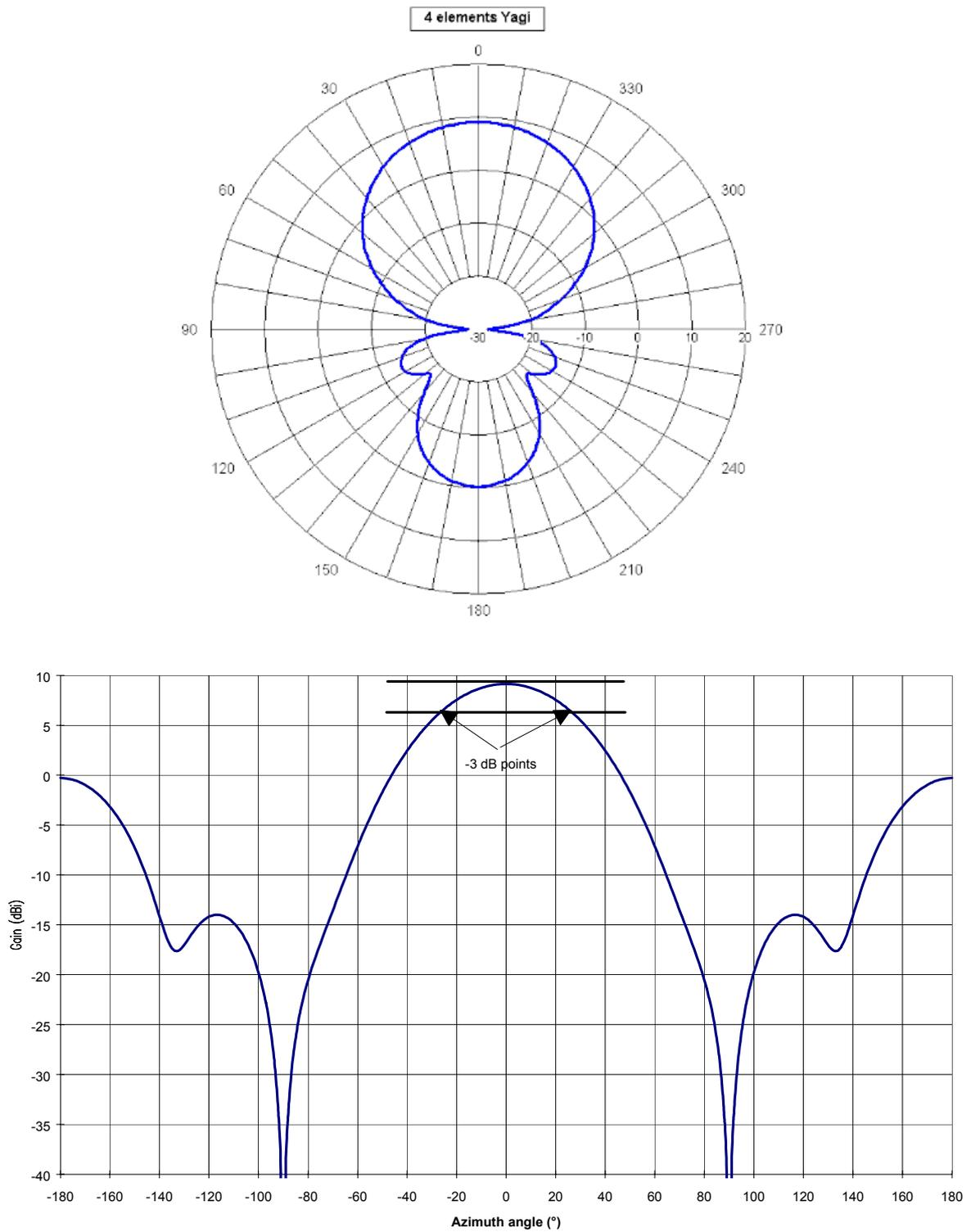
**Figure 3-5 Polar diagram (top) and rectangular diagram (bottom) of same antenna pattern**
