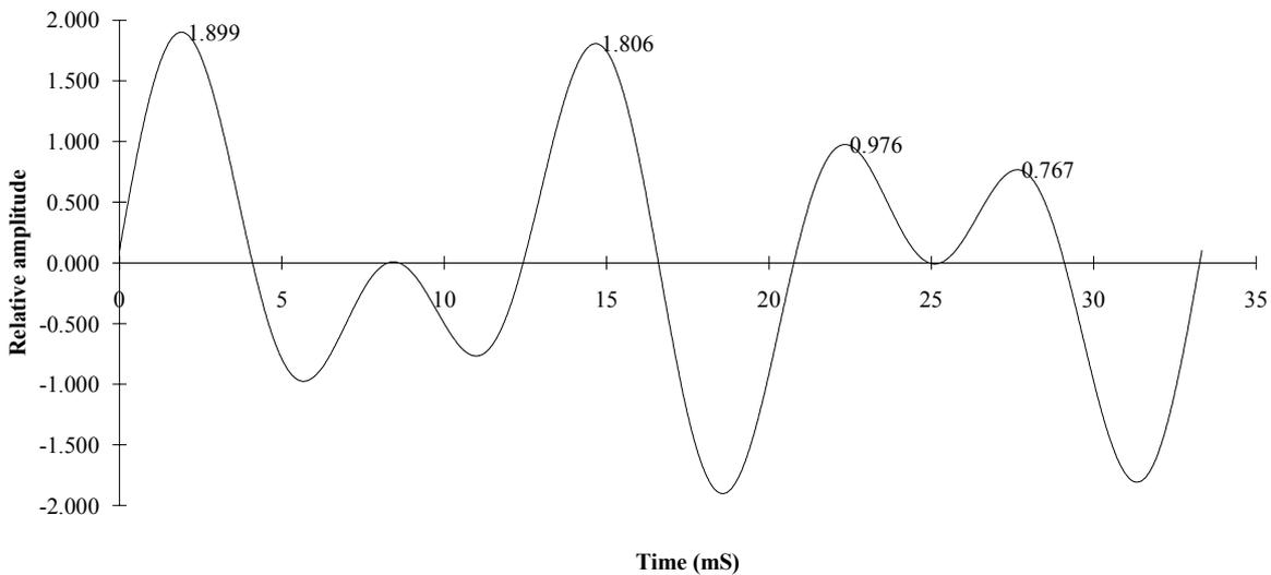
**Figure B - 2 +10° phase error (90 Hz) in reference to 150 Hz, and the resulting envelope**
