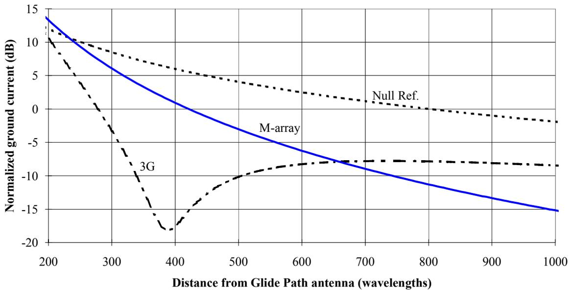
**Figure C- 1 SBO ground current distribution**
