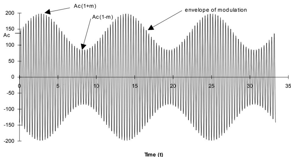
**Figure 2-3 An amplitude modulated signal**
