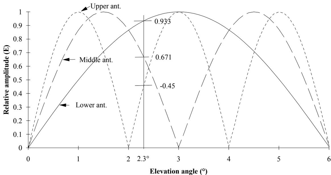
The monitor network should include the above given attenuation values for Middle Antenna (2.9 dB) and Upper Antenna (6.3 dB) referenced to Lower Antenna (0 dB). The signal path must also include a delay of 180° for Upper Antenna return signal.
