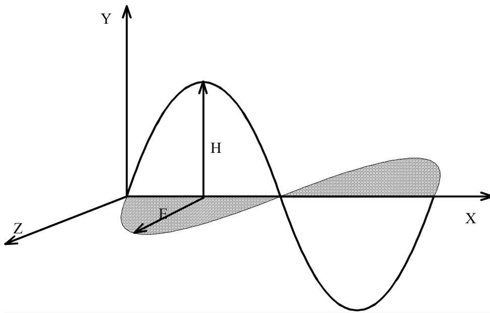
**Figure 3-1 Electromagnetic wave with E- and H-field lines**
