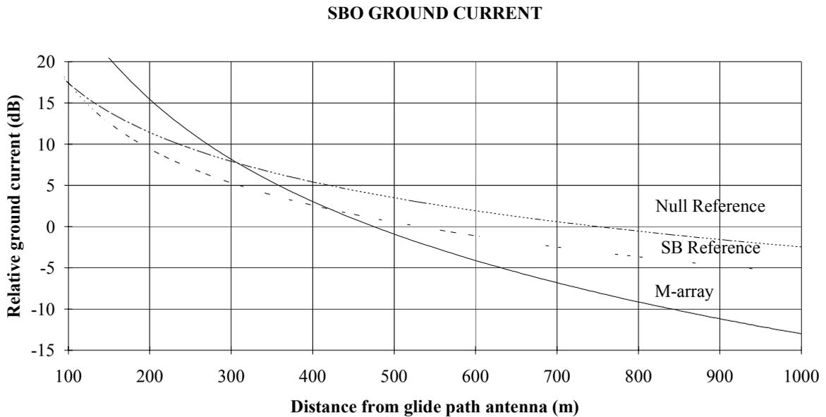
**Figure 6-21 Relative SBO ground current referenced to the critical level 0 dB**
