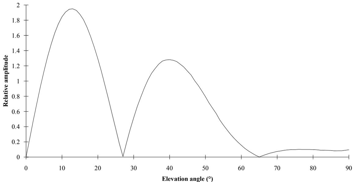
**Figure 4-4 Vertical radiation pattern of LPDA 3 m above ground**
