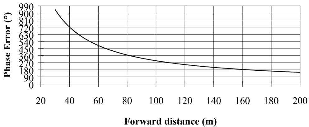
**Figure 7-4 The phase error vs. the distance to the antenna system for Null Reference, Sideband Reference and M-Array antenna systems**
