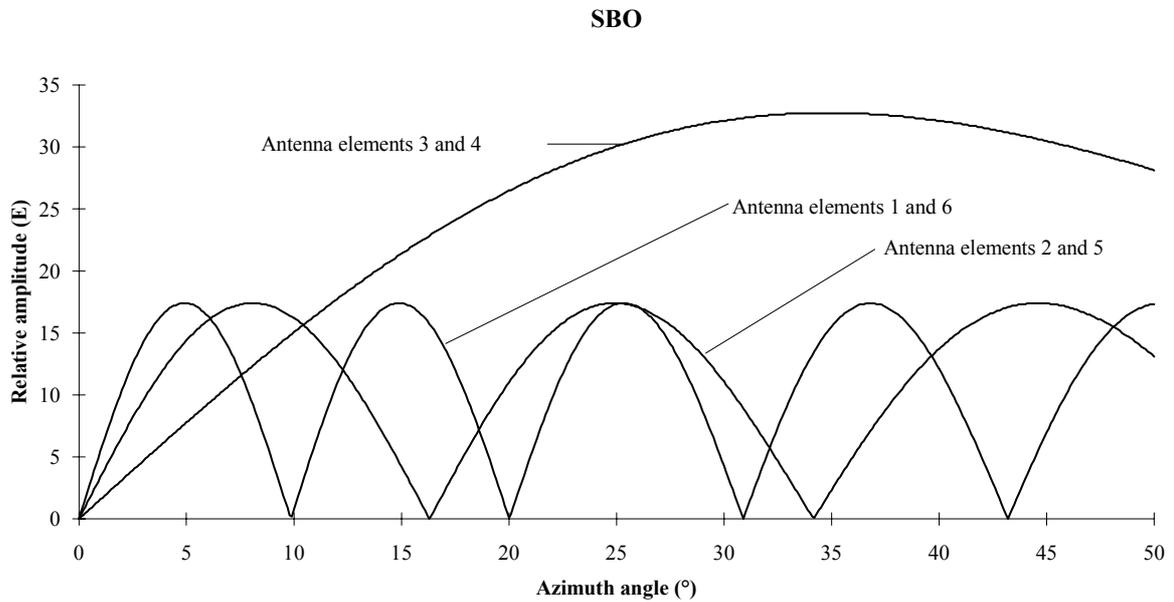
**Figure 5-2 CSB and SBO radiation patterns of the three antenna element pairs.
