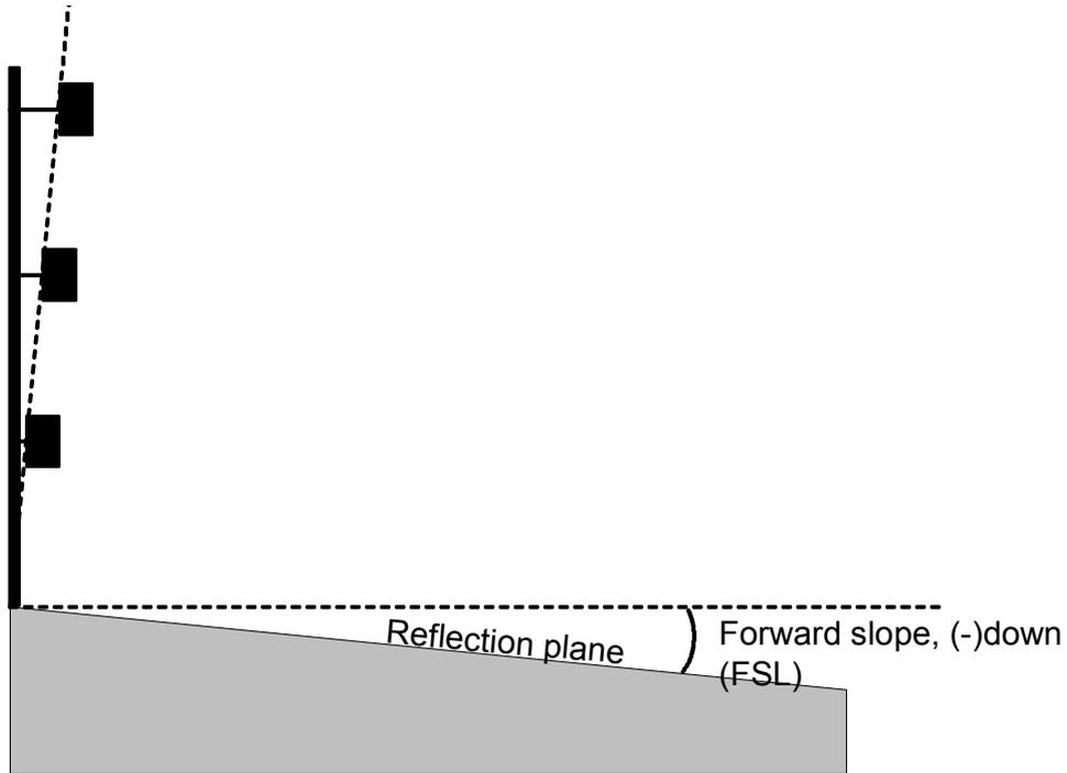
**Figure 6-19 Definition of Forward Slope (FSL)**
