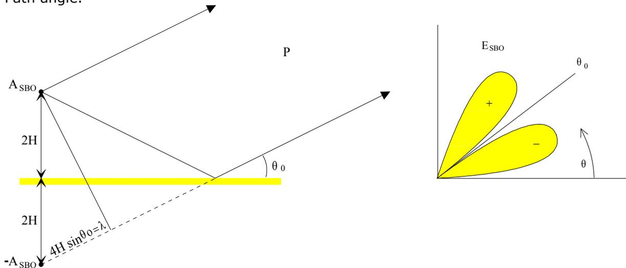
**Figure 4-11 Antenna element fed with SBO signal producing a null in the radiation pattern at  $\theta_0$**
