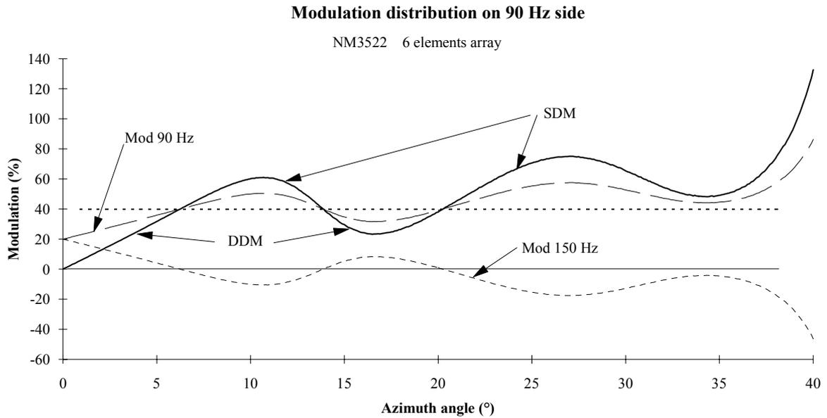
**Figure 5-4 Calculated DDM and modulation distribution
