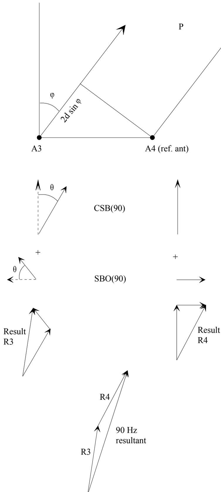
**Figure 4-1 Resulting 90 Hz sideband from two-antenna feeds**
