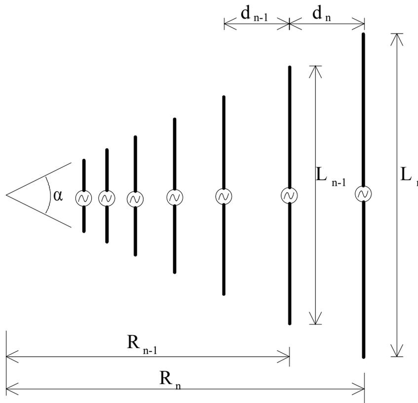
**Figure 4-6 LPDA with seven dipoles**
