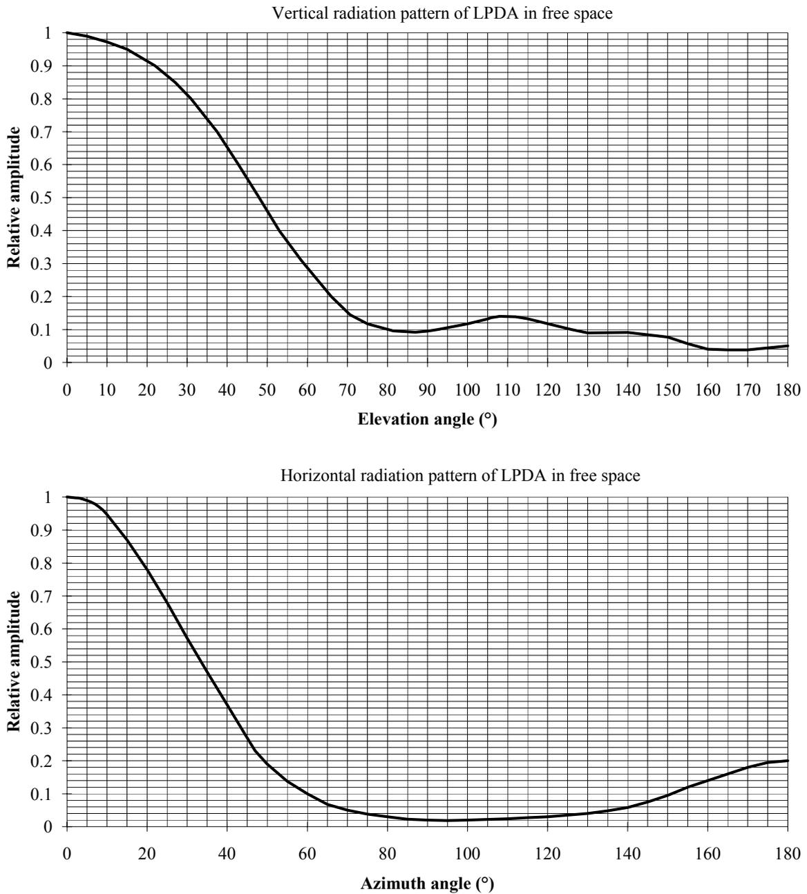
**Figure 4-9 Radiation pattern of the localizer LPDA**
