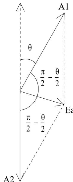
**Figure 3-10 Radiation from the elements fed  $180^\circ$  out of phase**
