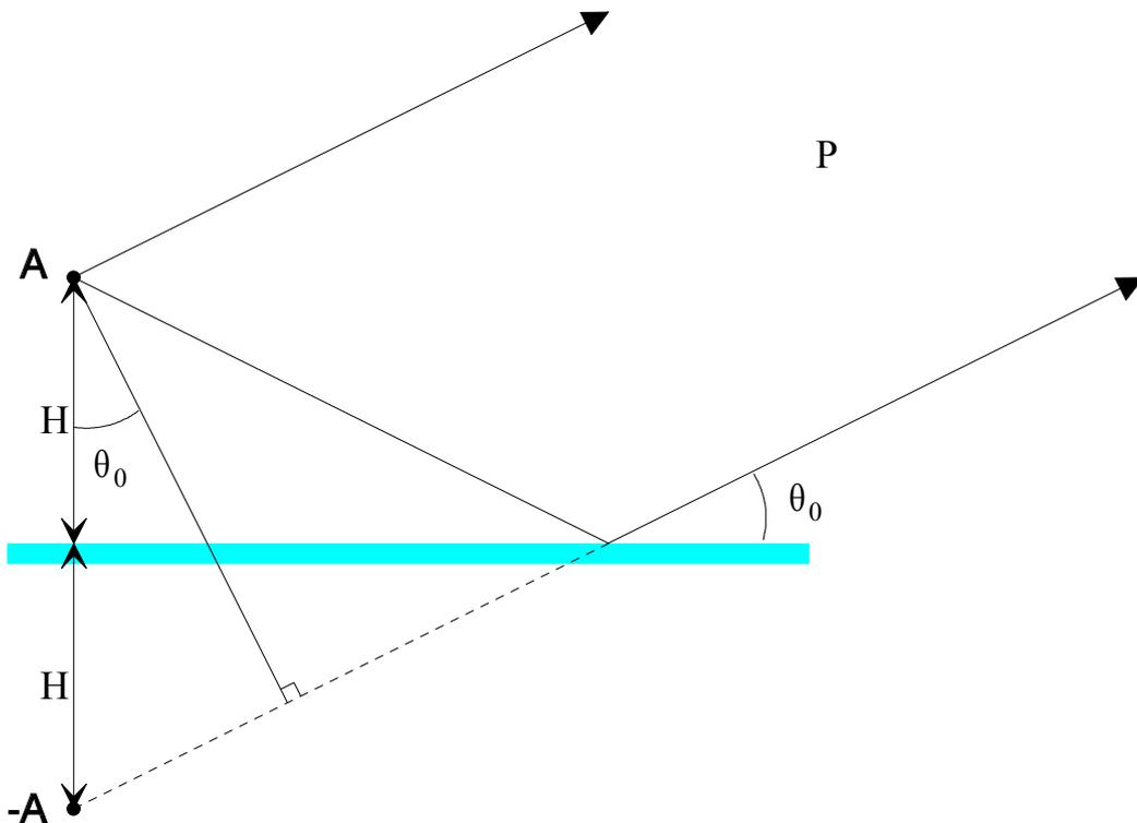
**Figure 4-10 Radiation from antenna above ground**
