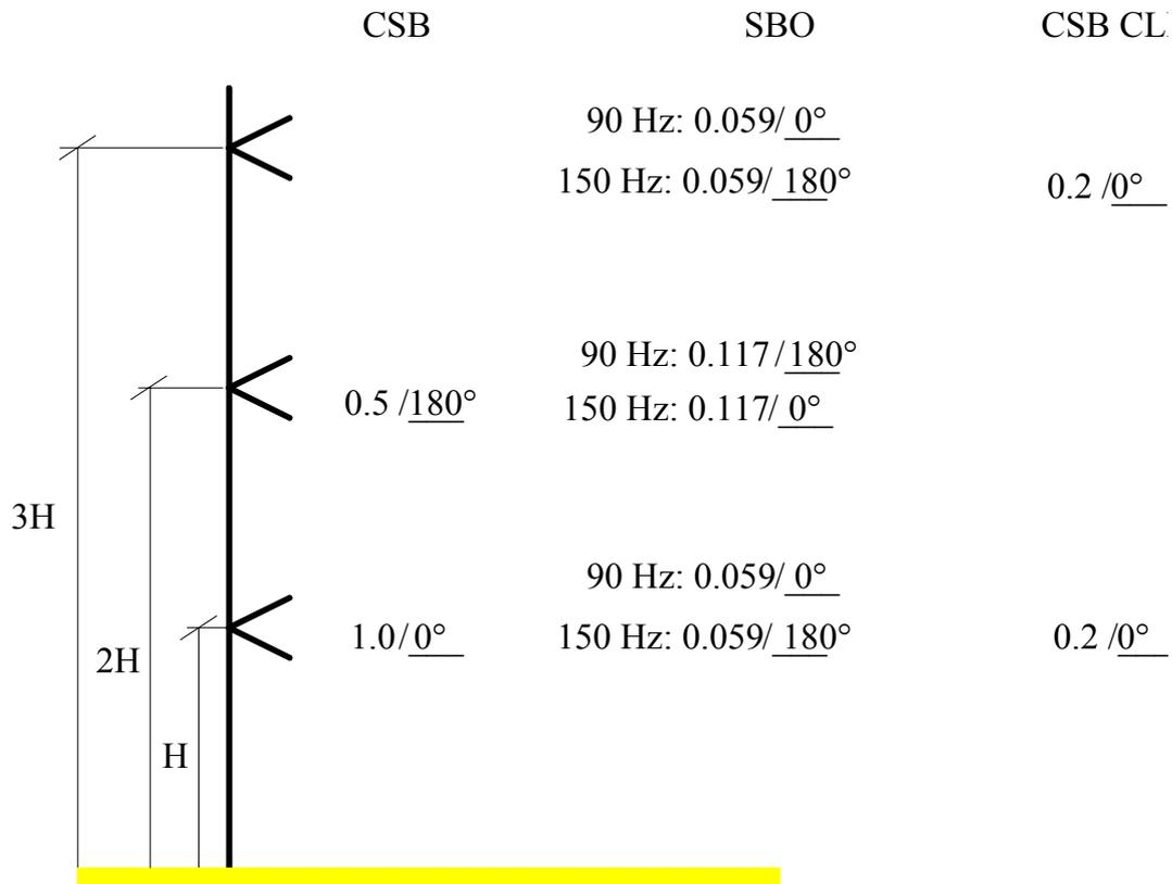
Figure 6-11 M-array Antenna Configuration
