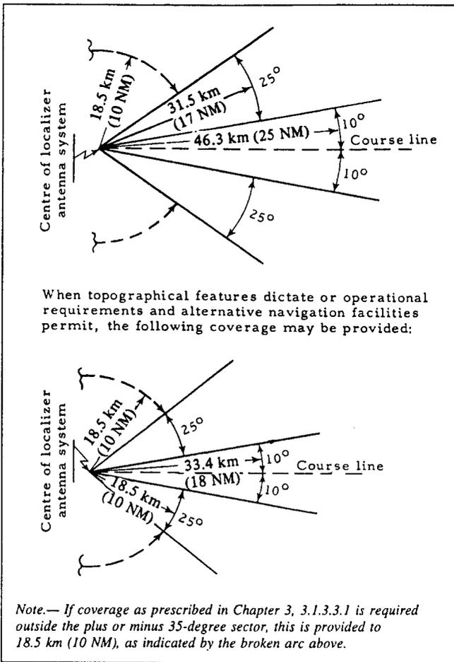
Figure C-7. Localizer coverage with respect to azimuth
