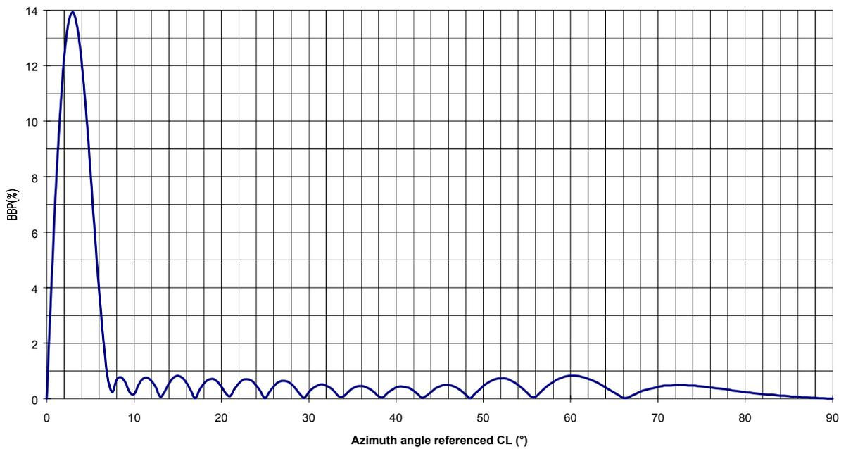
**Figure 5-22 Beam Bend Potential**
