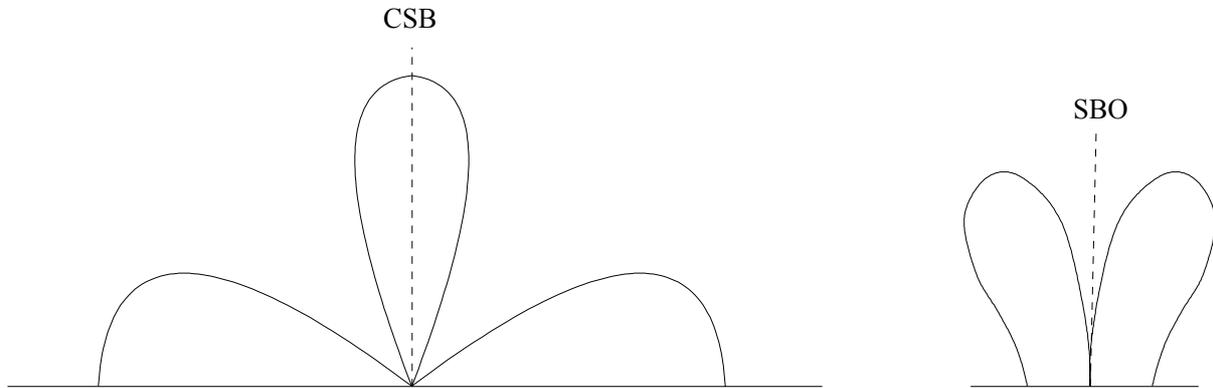
**Figure 4-3 Two antennas radiation patterns in polar coordinates for CSB and SBO feeds. Distance between antennas  $0.87\lambda$**
