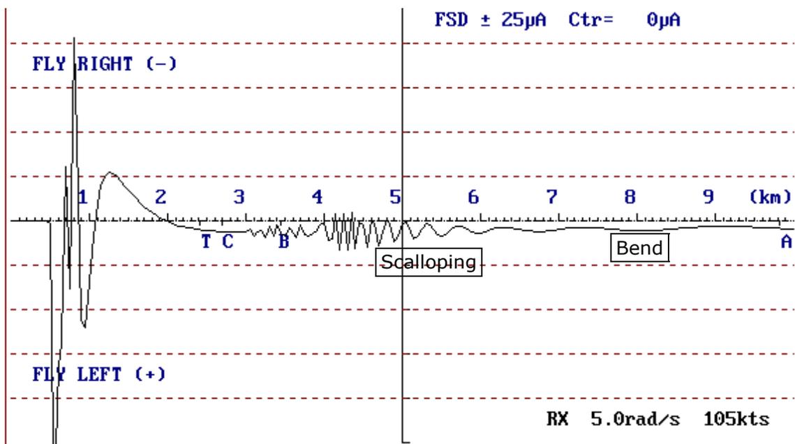
**Figure 8-1 Roughness, scalloping and bend on the course structure**
