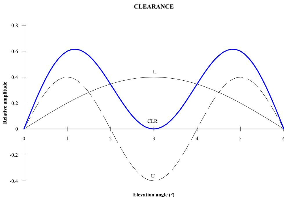
Figure 6-17 M-Array Clearance Far Field Radiation Pattern
