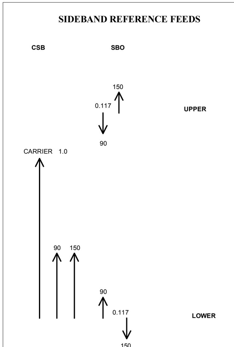
**Figure 6-10 Vector representation of Sideband Reference feed signals**
