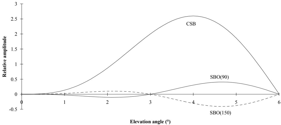
**Figure 6-14 CSB and SBO radiation pattern for M-array System**
