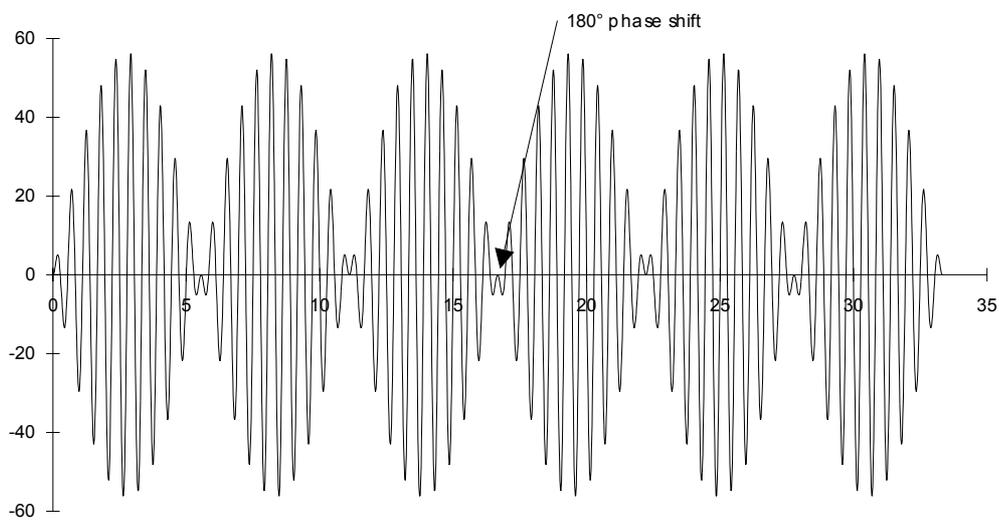
**Figure 2-6 A DSB - SC signal modulated with 90 Hz**
