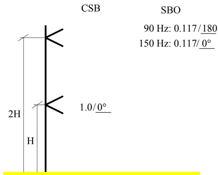
**Figure 6-1 Null Reference Antenna Configuration**
