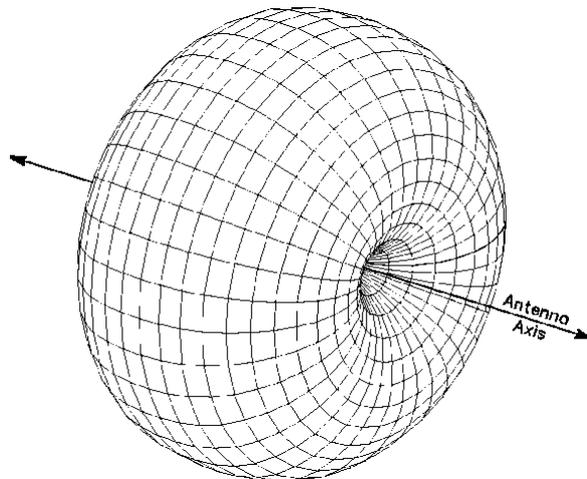
Figure 3-4 Omni directional Radiation Pattern
