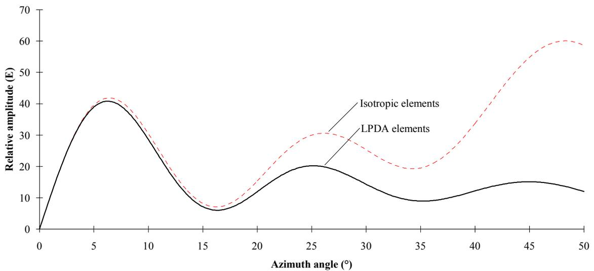
**Figure 5-3 CSB and SBO radiation patterns with and without the pattern of the LPDA included. (CS = 5°)**
