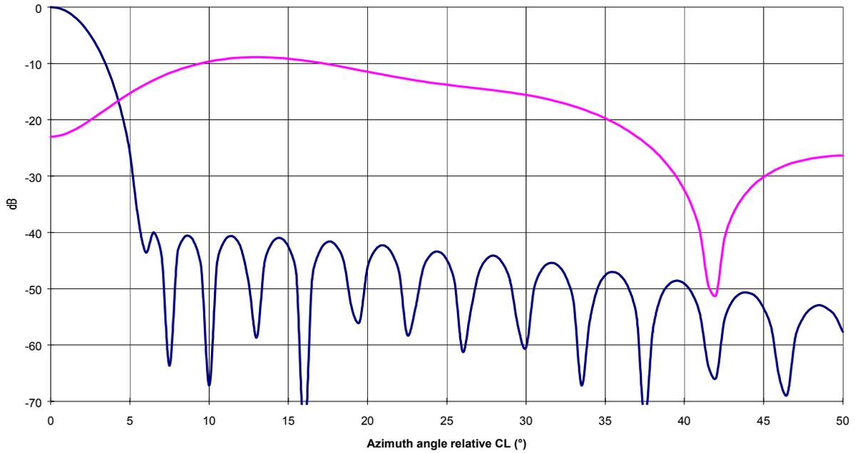
**Figure 5-14 Antenna Course and Clearance lobing**
