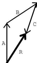
Figure 2-2 Graphic phasor addition of three signals
