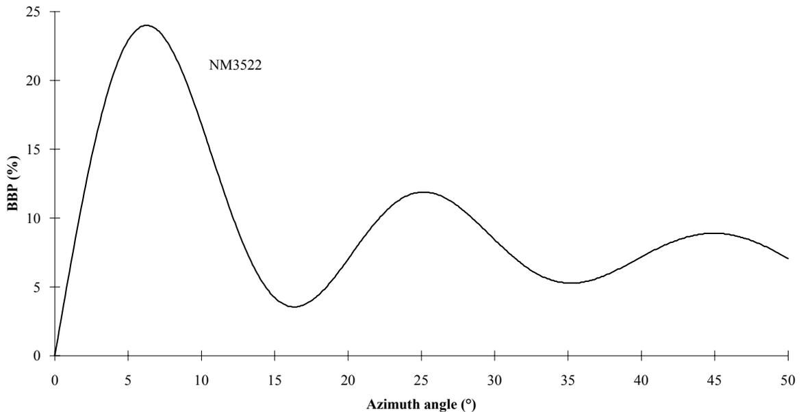
**Figure 5-5 BBP( $\varphi$ ) for CS = 5°,  $\varphi$  is the direction to the reflecting object**
