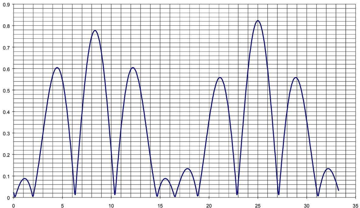
**Figure 2-19 Demodulated SBO with 0.2 dB unbalanced C+SB90 and C+SB150**
