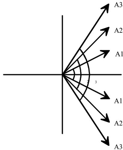
**Figure 3-12 Six Elements Antenna Array fed in-phase, and associated radiation vectors**
