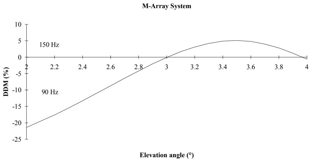
**Figure 7-7 DDM distribution at 82 m from the antenna system**
