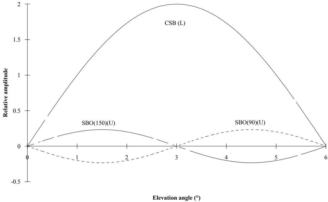
**Figure 6-2 CSB and SBO lobe patterns for Null Reference antenna system**
