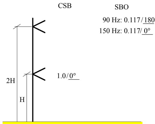
**Figure 4-12 Null Reference Antenna System**
