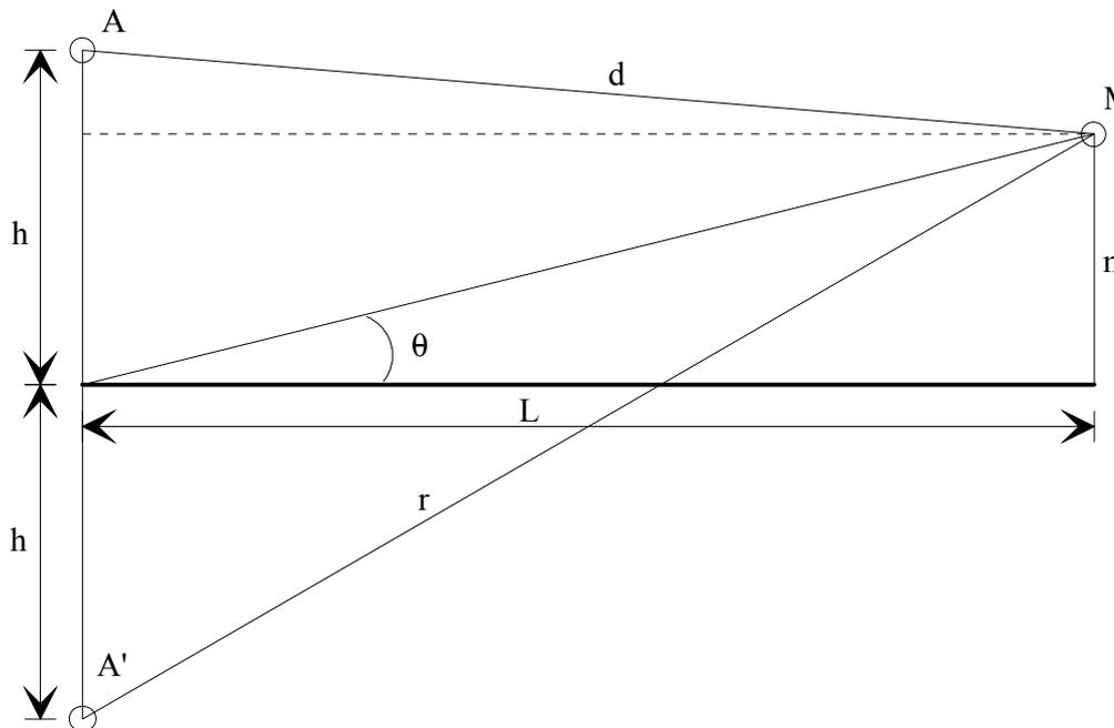
**Figure 7-2 Path lengths from an Antenna element A and it's Image A' to a Monitor point M**
