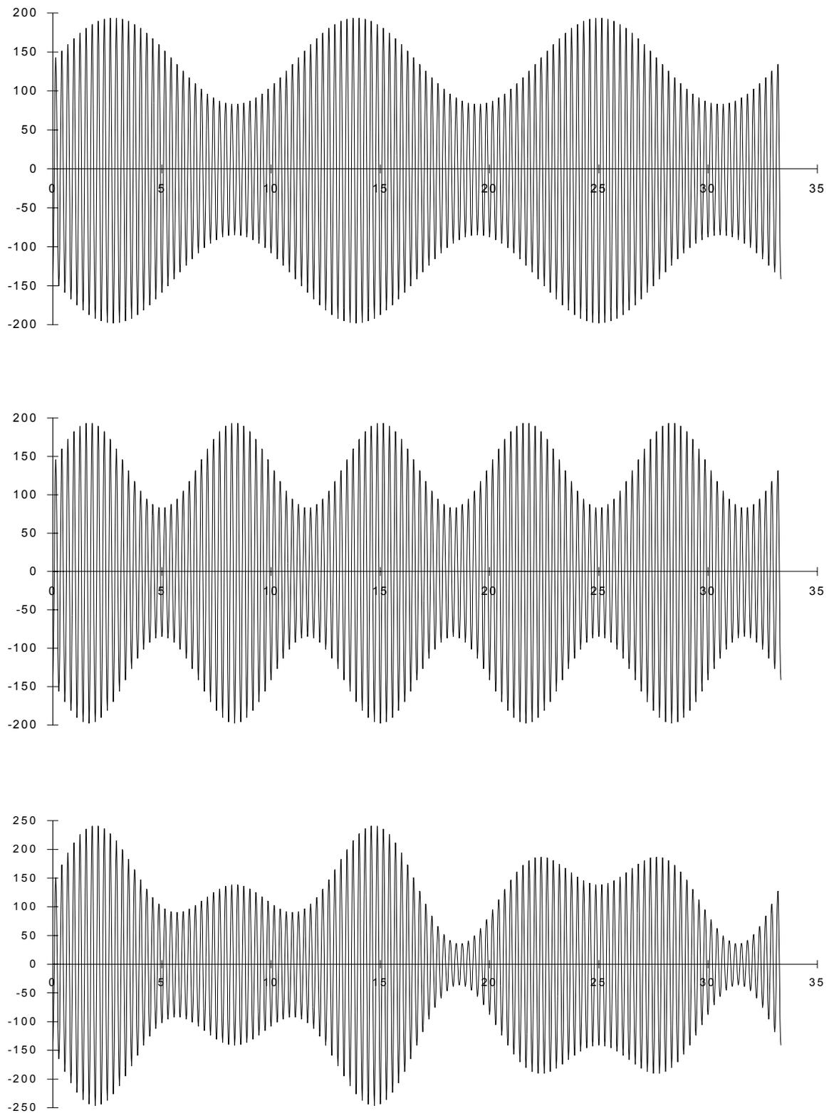
**Figure 2-8 The CSB waveform seen in the time domain. Upper diagram is 90 Hz, middle is 150 Hz, and lower is combined 90 + 150. Time scale in milliseconds**
