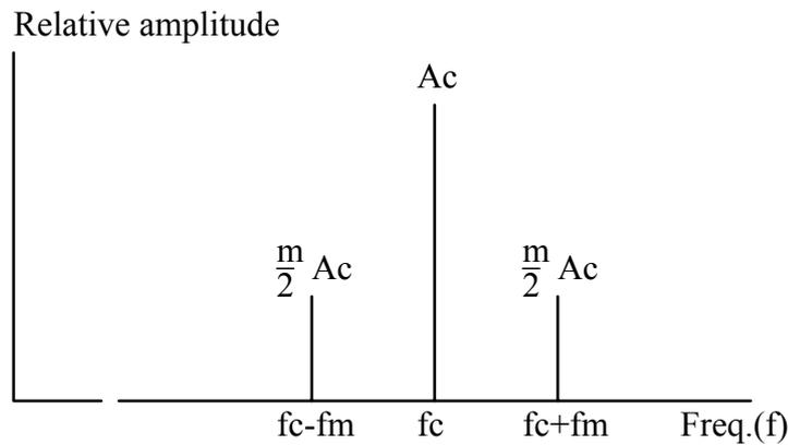
**Figure 2-4 The frequency spectrum of an AM signal**
