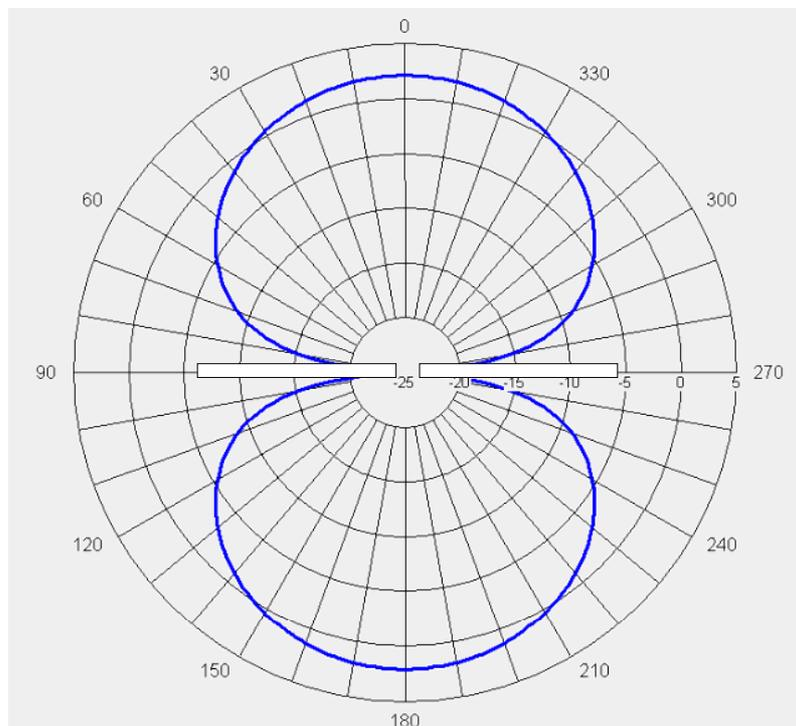
**Figure 3-7 Radiation pattern of a  $\lambda/2$  Dipole antenna in the plane of the dipole**
