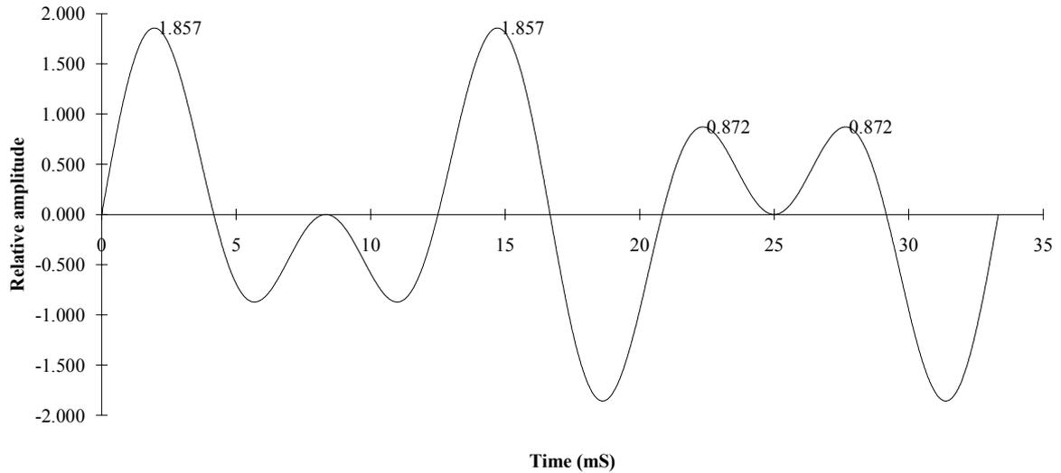
**Figure B - 1 Perfect 90 Hz and 150 Hz modulation tones and envelope, zero phase start point.**
