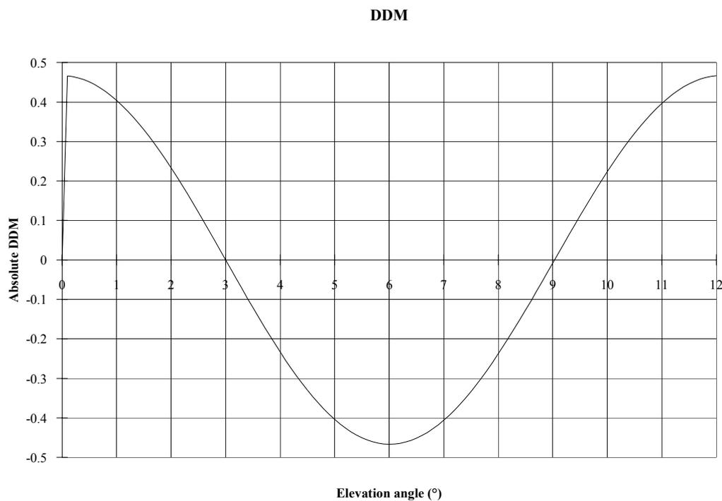
**Figure 6-9 The DDM distribution with normal feeding**
