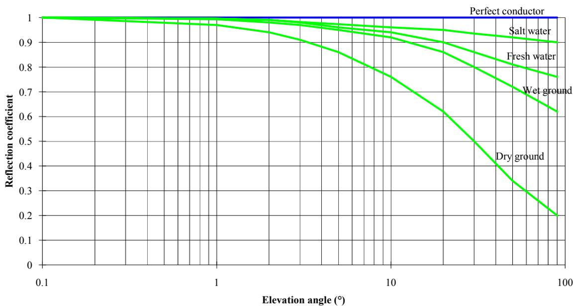
**Figure 4-5 The reflection coefficient for different materials**
