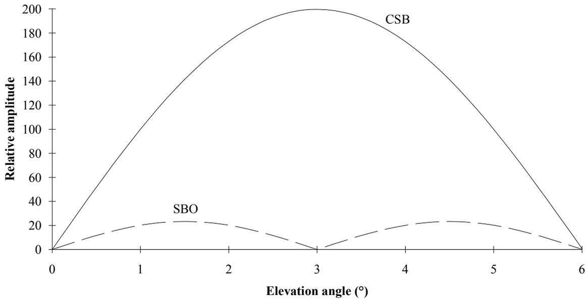
**Figure 4-13 CSB and SBO radiation pattern for Null reference Antenna System**
